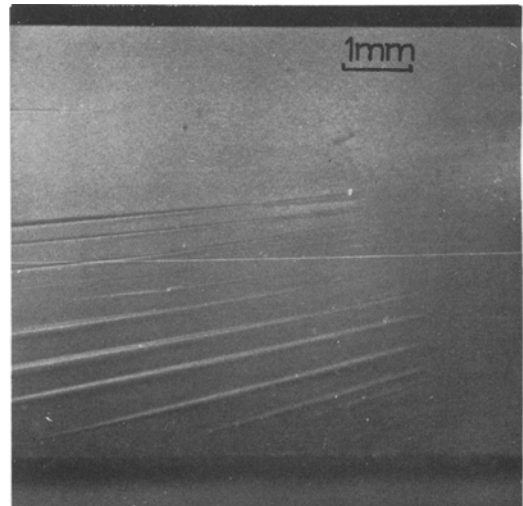
Figure 3 Fracture surface of an unexposed, notched resin cast fracture toughness specimen.
